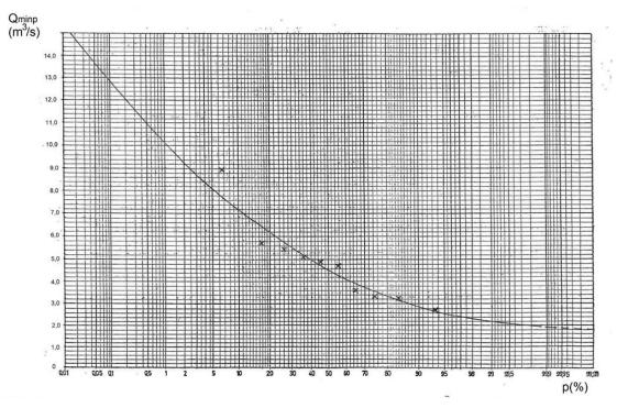
**Figure 4.24:** Minimum annual discharges with different return periods for the Klokot at the Klokot profile  $Q_{minp}$  (Type-III Pearson)  $Q_{minav} = 4.79 \text{ m}^3/\text{s}$ ;  $c_v = 0.36$ ;  $c_s = 1.14$
