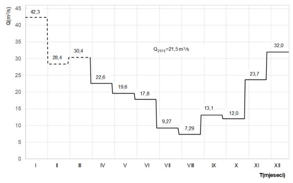
Figure 4.16: Hydrograph of the Klokot mean monthly discharges at the Klokot profile in 2010
