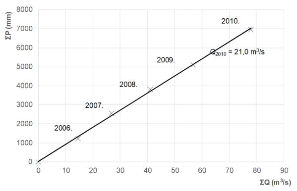
**Figure 4.7:** Double-mass analysis of the Klokot mean annual discharges at the Klokot profile  $\Sigma Q$  and annual precipitation at the Bihać Weather Station  $\Sigma P_B$  for the period (2006-2010)
