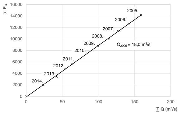
**Figure 4.9:** Double-mass analysis of the Klokot mean annual discharges at the Klokot profile  $\Sigma Q$  and annual precipitation at the Bihać Weather Station  $\Sigma P_B$  for the period (2005-2014)
