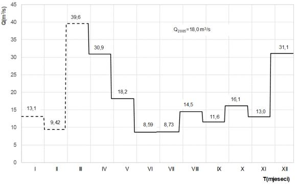
Figure 4.11: Hydrograph of the Klokot mean monthly discharges at the Klokot profile in 2005
