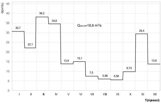
Figure 4.19: Hydrograph of the Klokot mean monthly discharges at the Klokot profile in 2013
