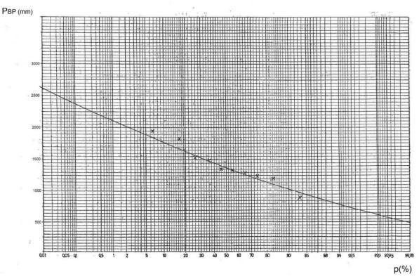
**Figure 4.10:** Annual precipitation with different return periods at the Bihać Weather Station  $P_{Bp}$  (Type-III Pearson distribution)  $P_{Bav} = 1,417$  mm;  $c_v = 0.20$ ;  $c_s = 0.21$
