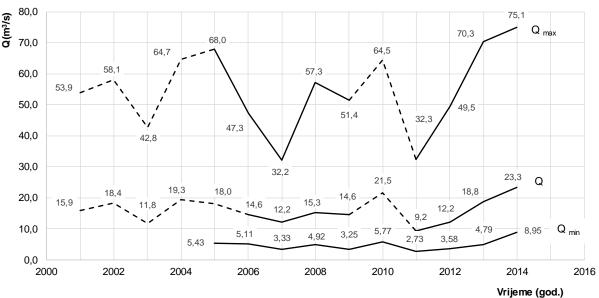
**Figure 1.1**: Maximum  $Q_{max}$ , mean Q and minimum  $Q_{min}$  annual discharges of the Klokot at the Klokot profile in the period (2001-2014)
