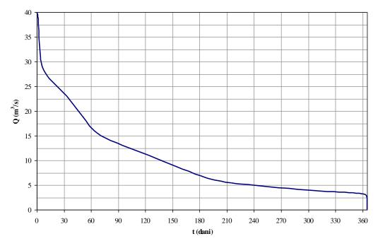
Mean daily flow-duration curve for the Klokot source for 1983 is given in Figure 4.2.
