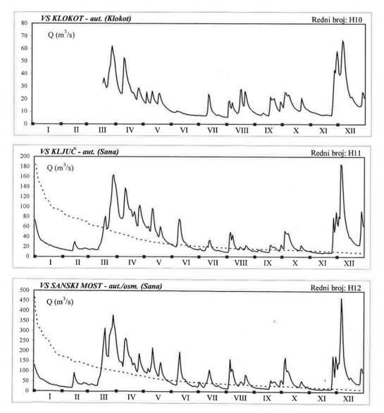
*Figure 4.3:* Hydrographs and flow-duration curves for the Klokot mean daily discharges at the Klokot profile and the Sana River at the Ključ and Sanski Most profiles in 2005 – Source: FMZ Hydrological Yearbook for 2005
