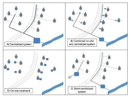
Figure 12.1: Different wastewater treatment systems
