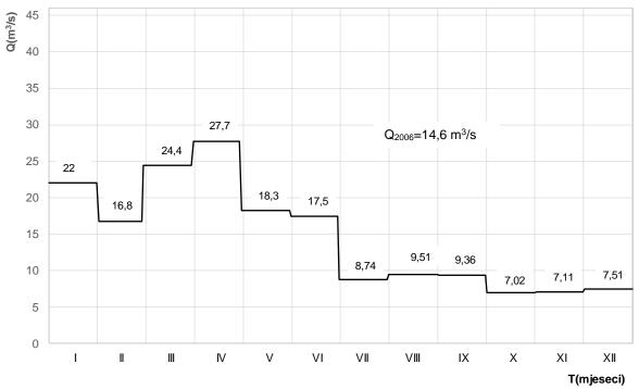
Figure 4.12: Hydrograph of the Klokot mean monthly discharges at the Klokot profile in 2006
