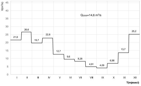
Figure 4.15: Hydrograph of the Klokot mean monthly discharges at the Klokot profile in 2009
