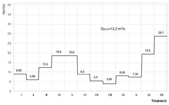
Figure 4.18: Hydrograph of the Klokot mean monthly discharges at the Klokot profile in 2012
