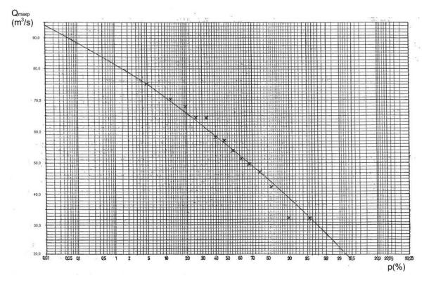
**Figure 4.23:** Maximum annual discharges with different return periods for the Klokot at the Klokot profile  $Q_{maxp}$  (Type-III Pearson)  $Q_{maxav} = 54.8 \text{ m}^3/\text{s}$ ;  $c_v = 0.23$ ;  $c_s = -0.31$
