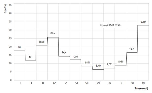
*Figure 4.14:* Hydrograph of the Klokot mean monthly discharges at the Klokot profile in 2008 – approximately average year for the period (2005-2014)
