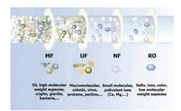
Figure 12.4: Ultrafiltration (UF) processes utilize a semi-permeable membrane to separate microcontaminants from a water stream.
