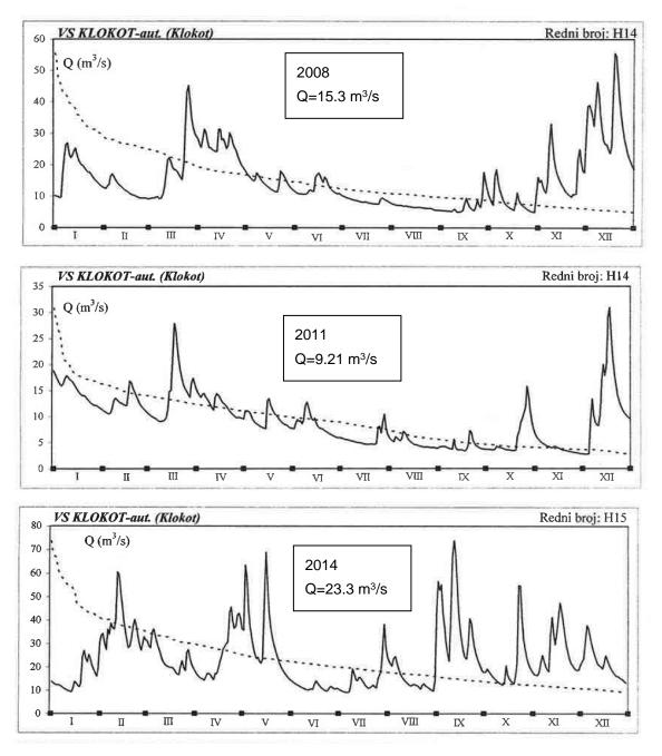
**Figure 4.21:** Hydrographs and flow-duration curves for the Klokot mean daily discharges at the Klokot profile in characteristic years: approximately average 2008, dry 2011 and humid 2014 – Source: FMZ Hydrological Yearbooks for 2008, 2011 and 2014
