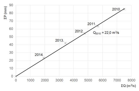
**Figure 4.8:** Double-mass analysis of the Klokot mean annual discharges at the Klokot profile  $\Sigma Q$  and annual precipitation at the Bihać Weather Station  $\Sigma P_B$  for the period (2014-2010)
