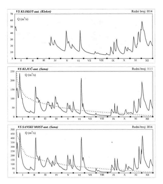
**Figure 4.4:** Hydrographs and flow-duration curves for the Klokot mean daily discharges at the Klokot profile and the Sana River at the Ključ and Sanski Most profiles in 2010 – Source: FMZ Hydrological Yearbook for 2010
