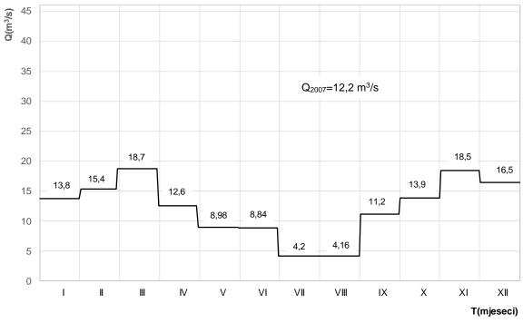
Figure 4.13: Hydrograph of the Klokot mean monthly discharges at the Klokot profile in 2007
