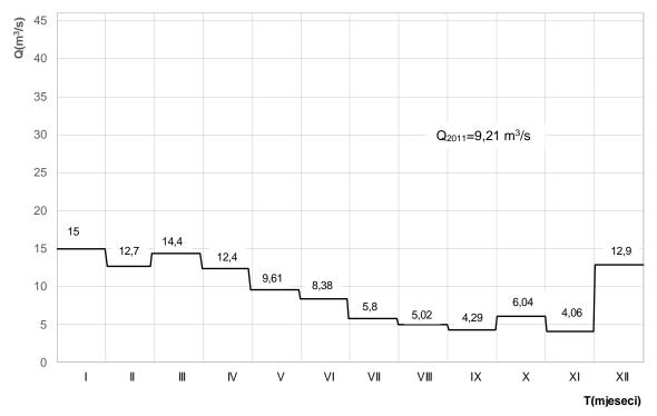
*Figure 4.17:* Hydrograph of the Klokot mean monthly discharges at the Klokot profile in 2011 – dry year in the period (2005-2014)
