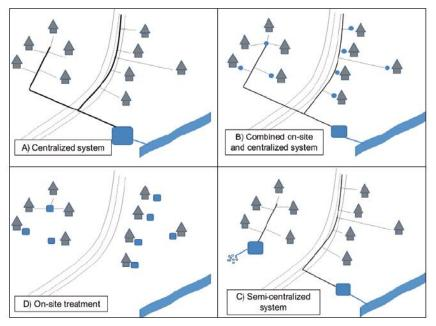
Figure 12.1: Different wastewater treatment systems
