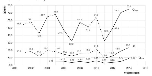
**Figure 4.25:** Maximum  $Q_{max}$ , mean Q and minimum  $Q_{min}$  annual discharges of the Klokot at the Klokot profile in the period (2001-2014)
