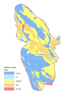
Figure 11.1: O factor (overlaying layers) - aquifer protective cover
