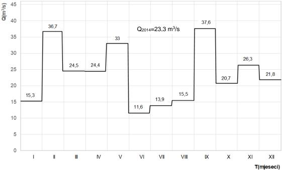
*Figure 4.20:* Hydrograph of the Klokot mean monthly discharges at the Klokot profile in 2014 – humid year in the period (2005-2014)
