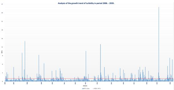
Figure 7.2: Variations of turbidity content between 2006 and 2020 in comparison with MAC values
