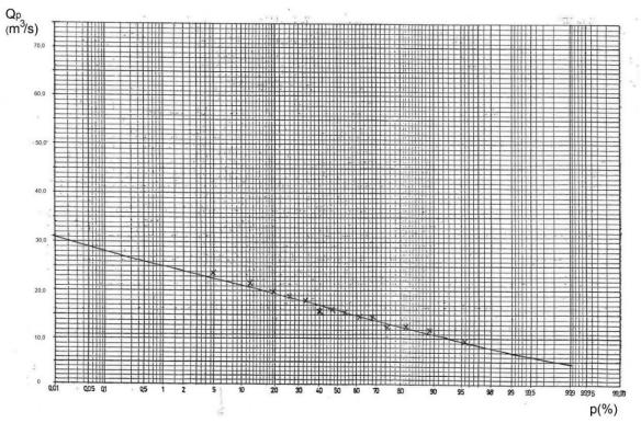
**Figure 4.22:** Mean annual discharges with different return periods of the Klokot at the Klokot profile  $Q_p$  (Type-III Pearson)  $Q_{av} = 16.1 \text{ m}^3/\text{s}$ ;  $c_v = 0.24$ ;  $c_s = 0.10$
