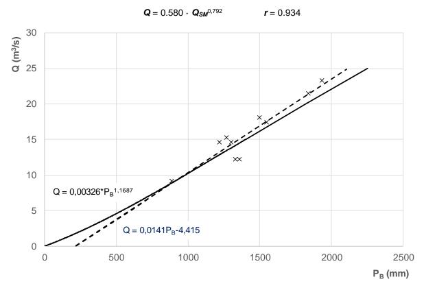
**Figure 4.5**: Correlation relationships (linear and nonlinear) between annual precipitation at the Bihać station  $P_B$  and the Klokot mean annual discharges at the Klokot profile Q
